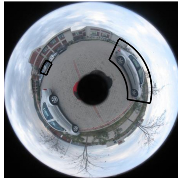
Fig. 3 Two cars in the omnidirectional image are indicated with black frames. The one close to the camera covers a larger area and it should be searched with a more bent sliding window, the other one is far away and it should be search with a more straight sliding window
