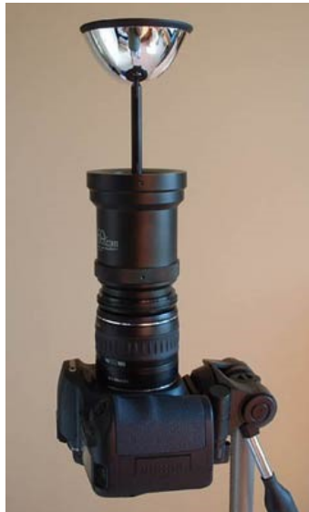
Figure 4.1. A mirror apparatus is placed in front of a conventional camera to obtain a catadioptric omnidirectional camera.
