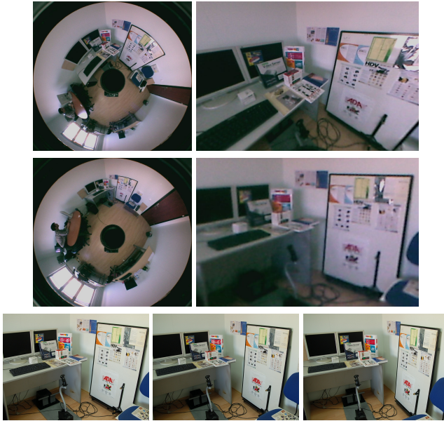
Figure 6: Images used for the experiment results of which is given in Table 2. Top row is Omni1 and VCP image generated from it (VCP1), second row is Omni2 and VCP2, bottom row is the perspective images, Pers1, Pers2 and Pers3. Omnidirectional images have a size of 1024x960 pixels, whereas perspective and VCP images are 1100x800 pixels. Please note that the hybrid image pair used in Table 1, Fig. 3 and Fig. 4 is Omni2-Pers2.
