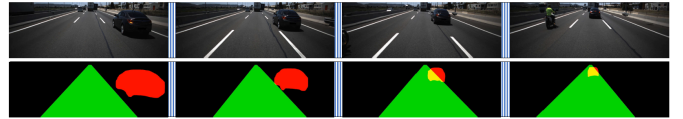
Fig. 3: The generation of a target-based scene representation is illustrated with an example of a left lane change maneuver from the Prevention Dataset. Distinct colors are used to illustrate overlapping masks of vehicles and the ego-lane. The figure presents four frames from a single sequence, while both the LSTM Network and the 3D network utilize 20 frames for classification purposes. The height of the video frames is reduced to 400 from 600 pixels to eliminate the hood of the ego-vehicle and a portion of the sky.
