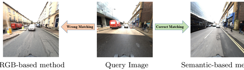
Fig. 4. An example query (middle) that RGB image method (left) fails but semantic descriptor (right) does not fail
