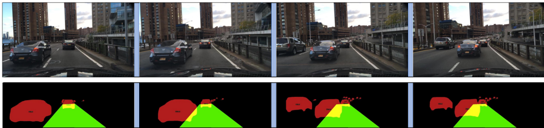
Figure 5.4. Generation of scene-based simplified view with an example cut-in maneuver from BDD-100K Cut-in/Lane-pass Subset. Overlapping masks of vehicles and ego-lane are in different colors. The figure shows four frames of a single sequence, whereas the 3D network uses 20 of them for classification. The frame height is reduced from 600 to 400 pixels to remove the ego vehicle’s hood and some sky.
